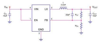
Adjustable Voltage Application Circuit
